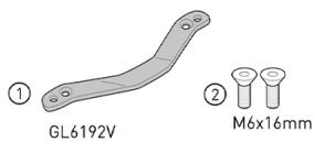
**Specific kit to install the specific rear rack KRA5143 on the original rack, offered as an option by the manufacturer**
