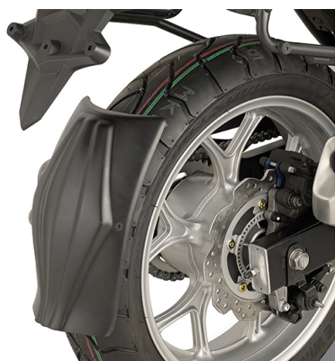
RM1146KITK Specific kit to install the spray guard KRM01, KRM02
